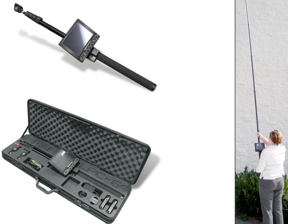
The camera head has built in variable illuminators providing crisp color images even in dark or low light situations. All controls are configured on the large (6.4 inch diagonal) color TFT monitor, providing a quick and easy-to-use inspection system right out of the case. The display monitor also provides a video output for other uses. Rechargeable battery packs (typical run time is between 1.5 – 2 hours) as well as a charger are included.
