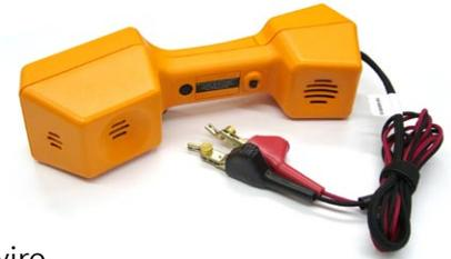
The most common type of phone amplifier is the traditional Butt-Set. Modern Butt-Sets often have features that include voltage readings and sometimes a simple TDR function that might tell you line length, but nothing more.
