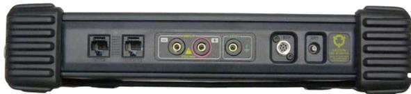
The Expansion port will be used for future upgrades. The RF Antenna port is used for RF broadband analysis using the 2 provided antennas.
