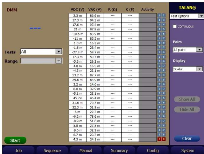
In this example, the resistance and capacitance were not measured because the line was actively connected to the switch. Resistance and Capacitance are only measured on an isolated dry line.
