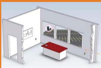
1. Capture a Friendly Reference Trace at a safe distance from the target sweep environment. Typically this can be done in the parking lot of the building at a reasonable distance from the Target Room. This Peak Trace is called the Friendly Trace. This data should be captured for at least 5 minutes, but better performance will be achieved by increasing the Friendly Capture time.
